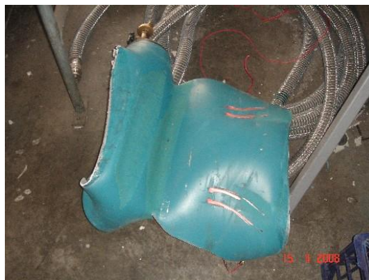
Ruptured incident cylinder weakened by exposure to heat and heat damage covered up by end user
